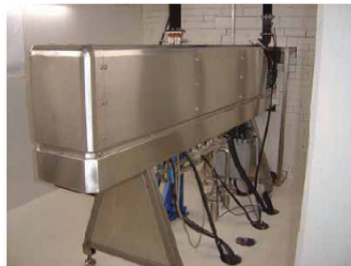
FIG.9. High power electron accelerator manufactured by Mevex, Sititville, Ontario,CANADA[37] IAEA Nuclear Energy Series No. NF-T-5.4 (2013)
